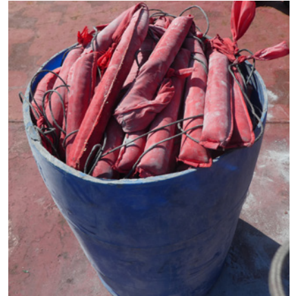
Exhausted fumigant residues in sleeves collected from the cargo surface can be a fire and health hazard
