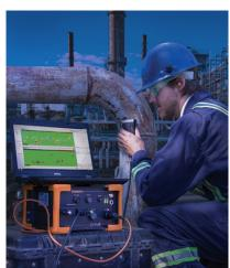
ECA is a natural extension of Eddy Current Testing (ECT) that improves on ECT technology by using multiplexed arrays of coils arranged in rows (instead of one or two coils). ECA can cover larger areas much faster and with greater sensitivity than ECT, using single scan passing to detect surface-breaking cracks as small as 0.5mm and sub-surface defects to a penetration depth of 6mm or more.
