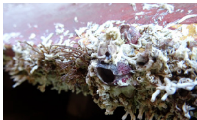
Barnacles, tubeworms, and soft fouling photographed on a ship's hull during drydocking survey
