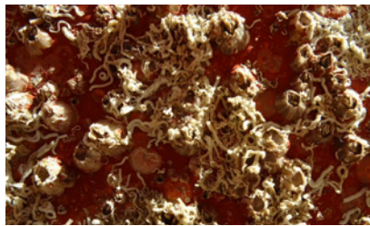
Barnacles and tubeworms photographed on a ship's hull during drydocking survey
