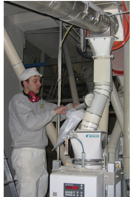
Diverter sampler in flour mill
