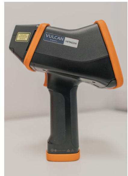
LIBS unit used for chemical analysis
