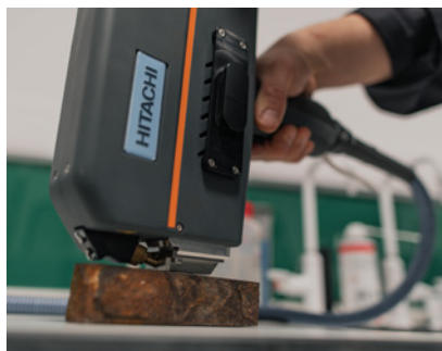
PMI OES unit used for chemical analysis
