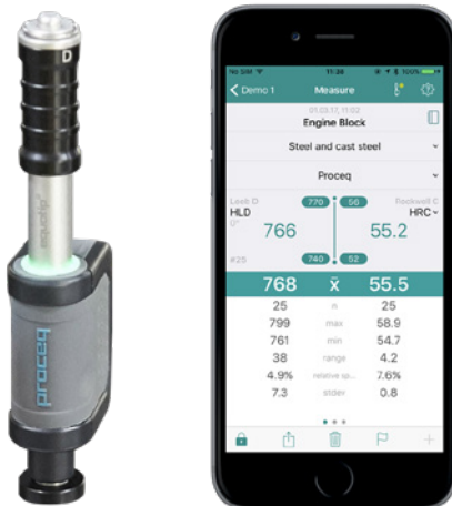
Portable Leeb D unit used for hardness testing
