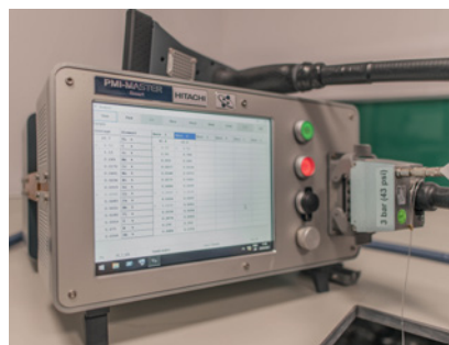
PMI unit displaying elemental data
