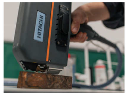
PMI unit for chemical analysis
