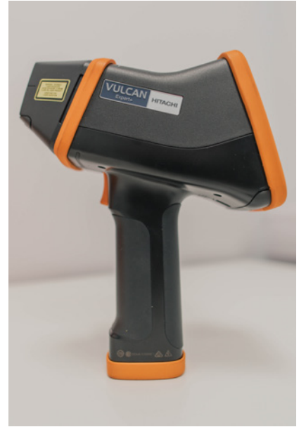
LIBS unit for chemical analysis
