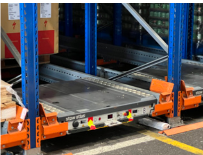
Typical racking types (Adjustable pallet racking and Pallet shuttle system) (Credit: PD Ports)
